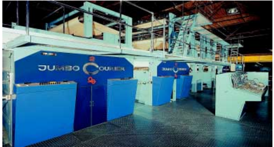
The Jumbo Courier six-by-four letterpress press of 1974 – a forerunner of today's superwide 6/2 KBA Commander offset giant
