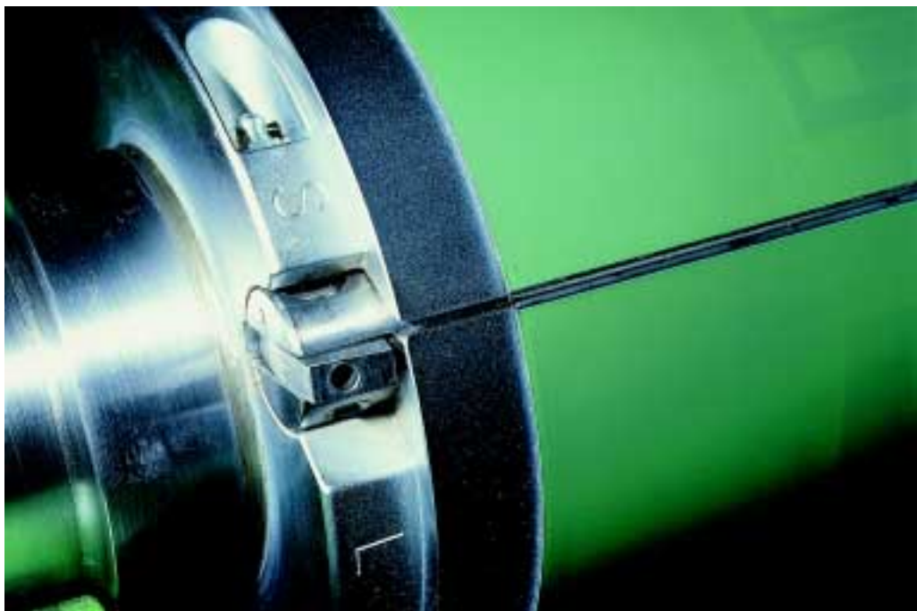
The minigaps and blanket plates launched by KBA in 1995, and now featured on more than 500 commercial printing couples, expand the options in newspaper offset
