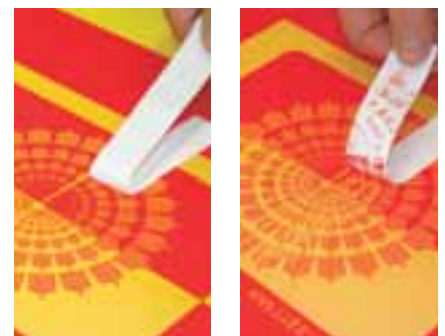
The adhesion test proves it: stencil material adheres very well; fine screen dots and lines stay firmly attached
